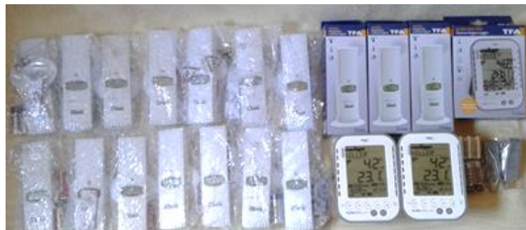
Figure 4. Internal units, thermo-hygrometer record transmitters and USB receivers.
