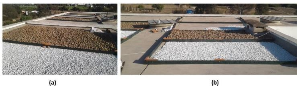
Figure 2. Materials used: (a) pebble parcel units, (b) gravel parcel units.
